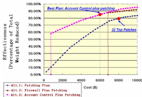
Figure 10 Optimal Security Practice Plan
